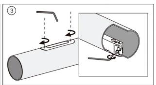
Suit for Standard Ø48-52mm round handrail wall thickness 0.8-3mm
