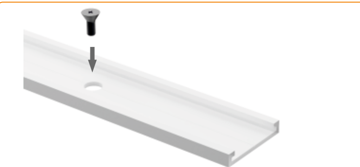
2. Mounting the RHEASCL-01A with screws
