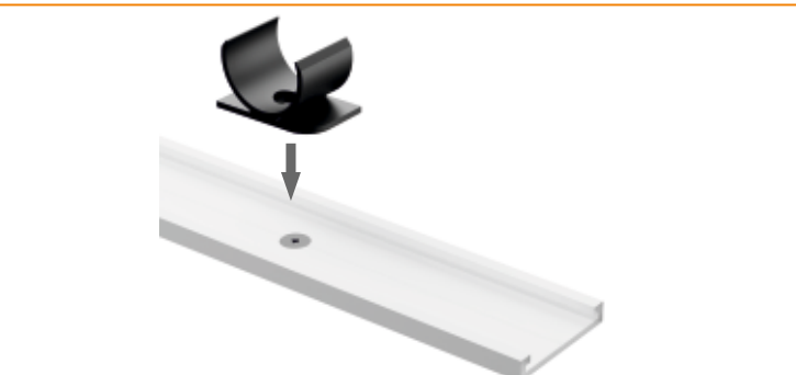
3. Install the mounting clips
